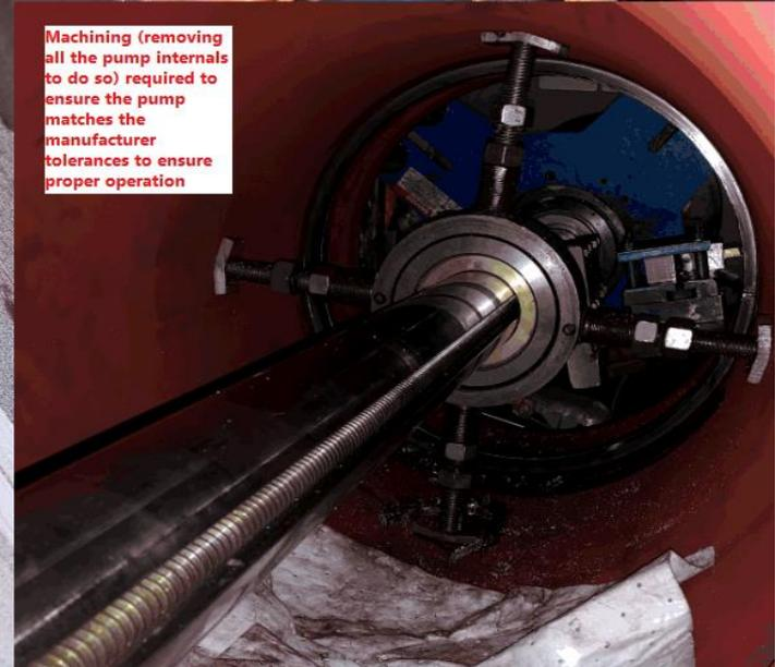
Machining (removing all the pump internals to do so) required to ensure the pump matches the manufacturer tolerances to ensure proper operation
